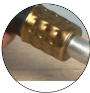
The die snaps quickly into the press fixture requiring no pins or screws.
