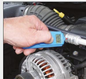
**52228 THERMOMÈTRE NUMÉRIQUE DE DIFFÉRENTIEL DE TEMPÉRATURE**
