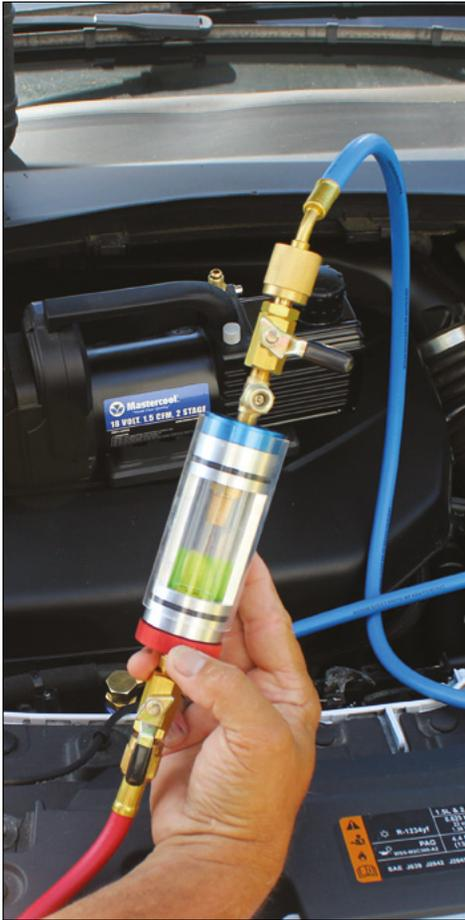
**GAGNEZ DU TEMPS EN DÉTERMINANT FACILEMENT SI LA CLIMATISATION DOIT ÊTRE RINÇÉE**
