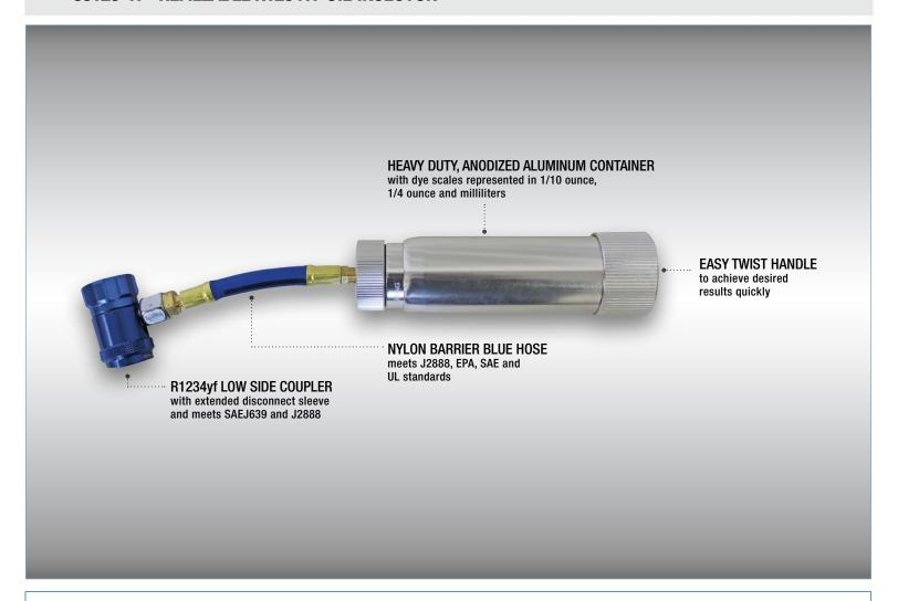
To inject the oil, simply connect the injector to the low side of the A/C system and twist the handle until you reach the desired amount. The injector hose comes complete with a R1234yf coupler.
