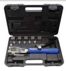
This kit fabricates factory style  $37^{\circ}$  and  $37^{\circ}$  double flare found on aviation and specialty automotive applications. The hand-held hydraulic pump operates easily with all steal and light stainless tubing. Includes: 3/16, 1/4, 5/16, 3/8 and  $1/2^{\circ}$  double flare adapters and  $37^{\circ}$  Cone.
